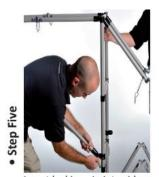
Insert locking pin into side support arm. Repeat steps 2-5 for the other half of rack. Make sure that all pins are secured.
