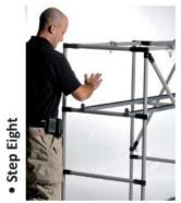
Insert long rollers on remaining tiers. Lightly tap rollers into position.
